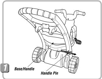
• If you are converting from the learn to pedal trike mode, remove the handle pin from the base/handle and the back of the frame.
